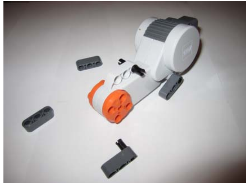
Step 2: Pin 1x3 Liftarms. Thread Long Pin with Friction
