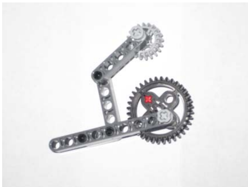
Step 3: Pin Gear 20 to Beam 5 and Bent 90
