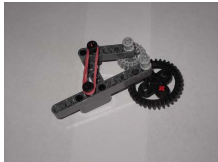
Step 4: Install Pin Long and loop with Rubber band
