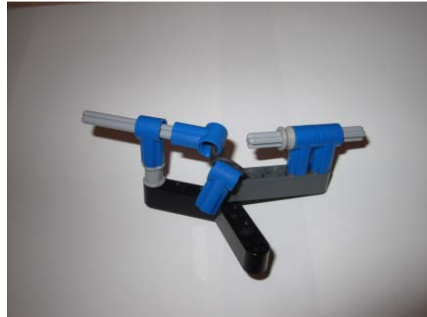
Step 4: Attach Connector #1s onto Axles
