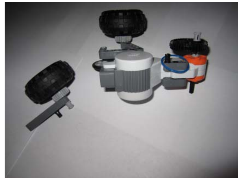
Step 4: Attach 36T Gears off-center. Attach Rubber Bands
