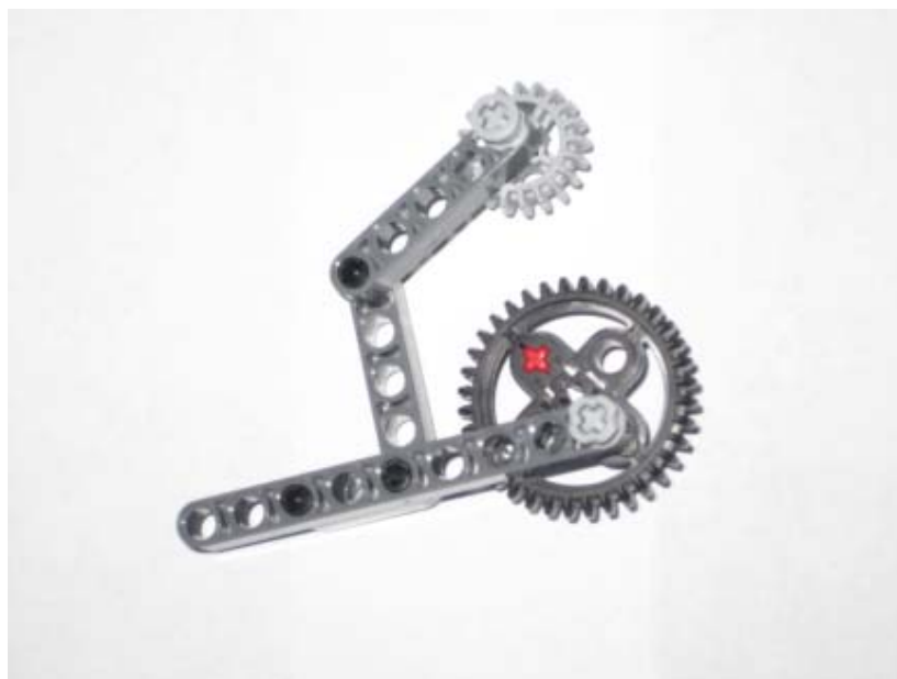
Step 3: Pin Gear 20 to Beam 5 and Bent 90
