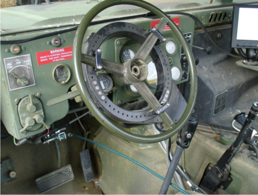
Steering Ring installed in a military HMMWV.
