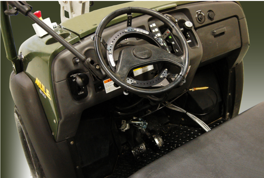
Steering Ring installed in a Kawasaki Mule.
