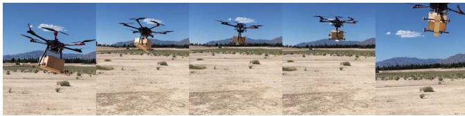
Fig. 3. UAV-UGV exhibits very unstable flight during yawing.
