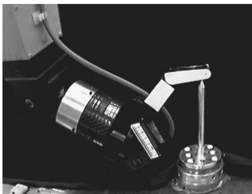
Figure 8: Finger of Barrett Hand applying force to instrumented probe
