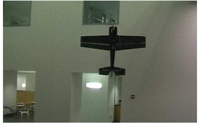
Fig. 7. MAV performing a *hands-off* autonomous hover in and urban structure.
