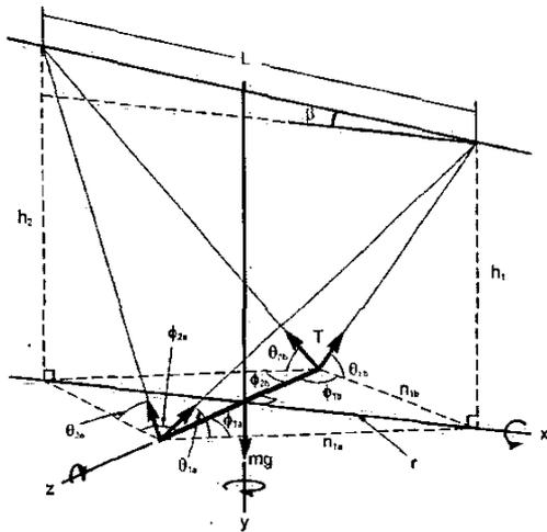
Figure 4: Small body force diagram for a Picavet
