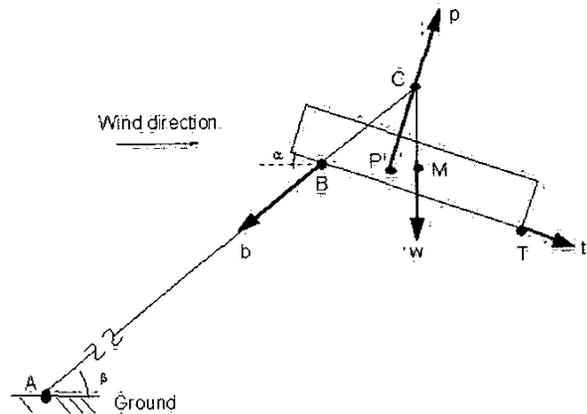
Figure 1: Simple kite model with forces in balance
