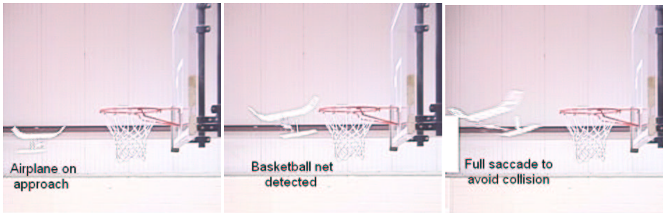
Figure 11. Optic flow is used to sense when an obstacle is within two turning radii of the aircraft. The aircraft avoids the collision by fully deflecting the rudder.
