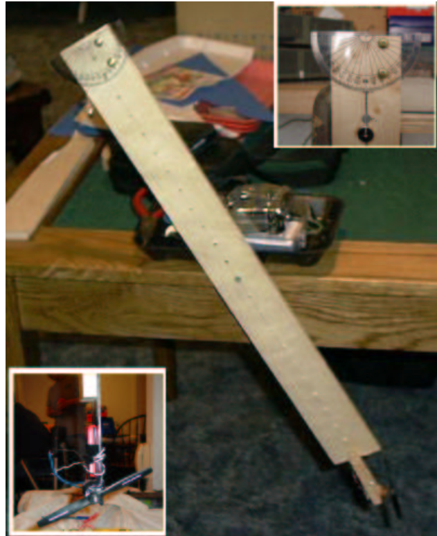
Figure 3: Lever arm angle as measured by the protractor (close up in upper right inset) is proportional to the rotational speed of the motor-propeller (close up in lower left inset). At equilibrium the dynamic thrust balances the torque due to gravity.
