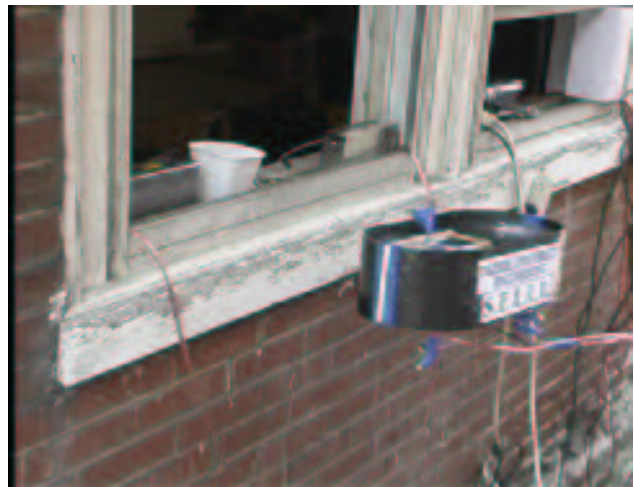
Figure 1: Backpackable aerial robot prototype with on-board camera performs hover-and-stare mission outside a window
