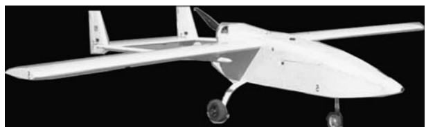
Fig. 9 The MAKO UAV developed by NAVMAR was modeled in X-Plane and used for experiment flights
