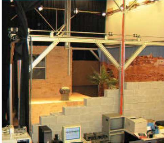
Figure 4: Systems Integrated Sensor Test Rig (SISTR). SISTR provides a stage for testing and evaluations of hardware to in simulated urban environments and disaster scenarios. Effects such as varied lighting, rain, fog and smoke can be introduced in a controlled and repeatable fashion.
