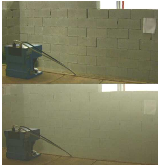
Figure 5: To characterize the SICK LMS200, the sensor was placed inside the testing environment and pointed toward a white sheet of paper placed 3m away. 500 data points were recorded without smoke (top) and in smoke with a visibility of approx. 15m (bottom).
