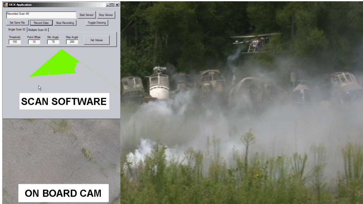
Figure 8: The LMS200 was attached to the bottom of the SR100 helicopter and flown over smoke. Results showed that the LMS200 reflected off of the smoke, but was still able to locate flat terrain to land.
