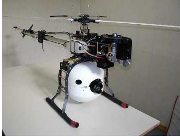
Figure 7: The SR100 robotic helicopter from Rotomotion, Inc. The SR100 is sold as a fully robotic package capable of automated take off, landing, and GPS waypoint following.
