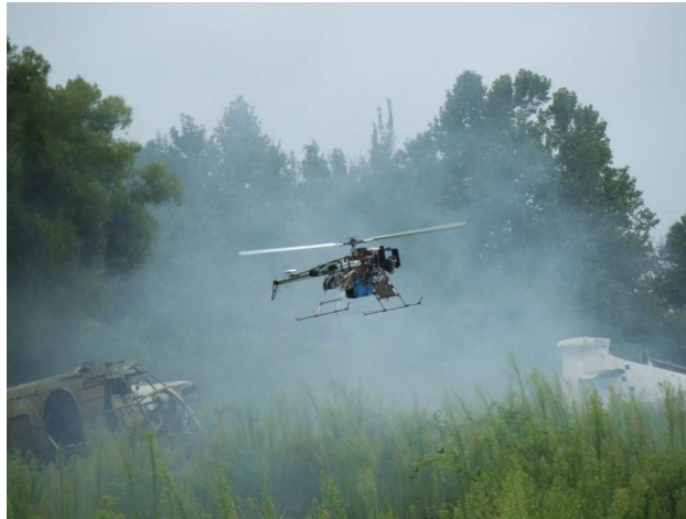
Figure 1: The SR100 robotic rotorcraft hovers over an unsafe landing site. A laser range finder mounted to the bottom of the craft is tested for its performance in smoke.
