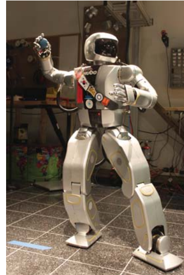
Fig. 1. Jaemi Hubo (Hubo KHR-4) demonstrating the initial pose for the overarching goal of creating a full body, human-like, stable, motion for throwing.
