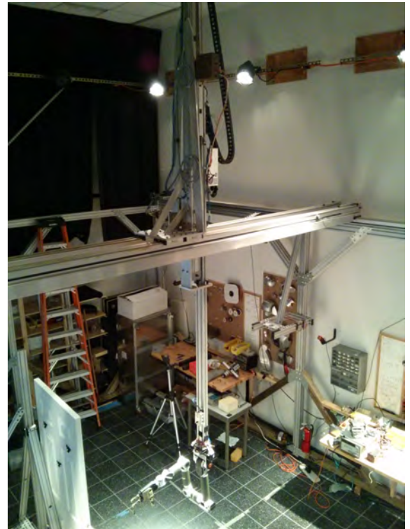
Fig. 3: MM-SISTR overhead gantry, gimbal, and manipulator
