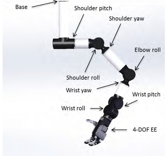
Fig. 4: CAD drawing of manipulator (showing each joint)
