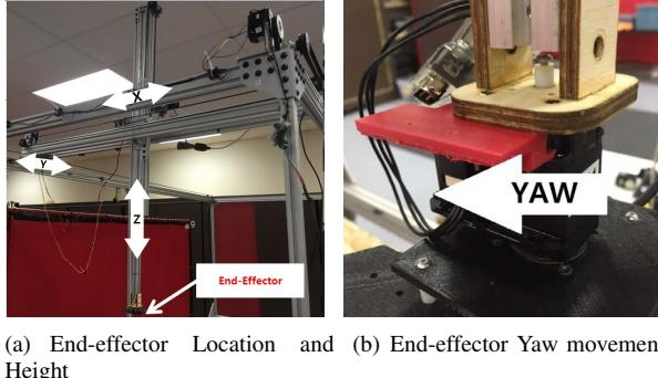
Fig. 3. The gantry crane system
