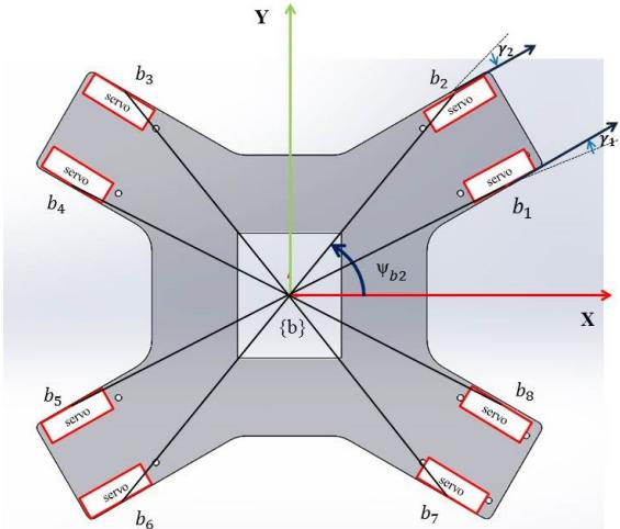
(b) Geometrical arrangement of leg attachment points
