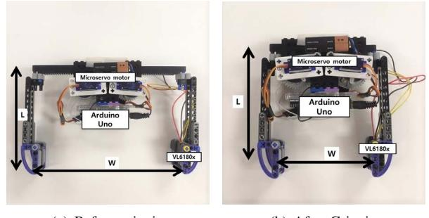
Fig. 5. LEGO-Based parallel gripper concept design
