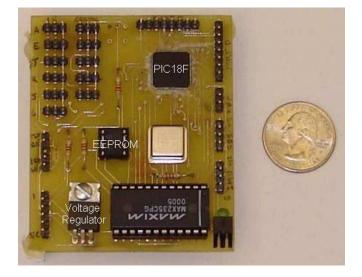
Fig. 6. Twenty-five-gram FCS was developed for controlling the hybrid prototype.
