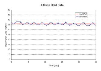
Fig. 16. Raw sonar data are plotted over the course of 20 s of fully autonomous hovering. The reference height value was set to 36 in. In the next 20 s, a board is placed under the aircraft to prove that the throttle is not set at a constant value to balance the aircraft weight.
