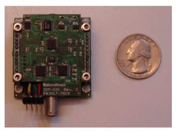
Fig. 5. Microstrain's 30-g IMU sensor was used to feedback attitude information to the onboard control system.
