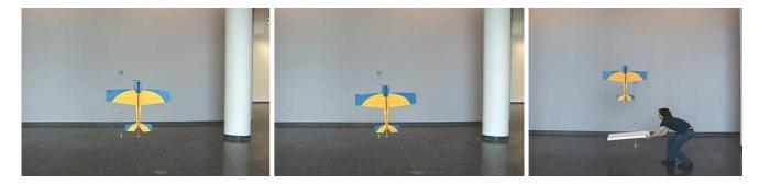
Fig. 15. First two images in the above sequence show the hybrid MAV in a fully autonomous hover at a height of 36 in at 6 s apart. In the third image, a board was placed under the MAV's tail that caused the controller to adjust the MAV's height to 36 in above the board. This was used to show that a constant throttle setting was not used to perform altitude hold.
