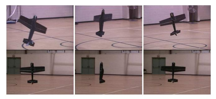
Fig. 8. (Top) Skilled human pilot hovers a fixed-wing aircraft in a small gymnasium and struggles to maintain a vertical orientation. (Bottom) Under autonomous control, the same aircraft is able to sustain a hover while remaining fixed in the vertical position.
