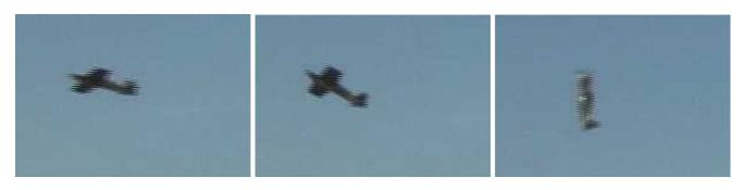
Fig. 10. Transition from (left) cruise flight, through (center) the stall regime, and into (right) hover mode is achieved autonomously.
