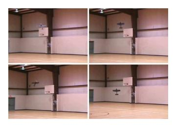
Fig. 11. (Top) Transition from cruise flight into hover mode is demonstrated inside an urban structure. (Bottom left) During the transition, the throttle is decreased to prevent the plane from colliding with the ceiling. This causes the aircraft to overshoot the vertical orientation. (Bottom right) The flight controller is able to recover and stabilize the MAV in its hovering orientation.
