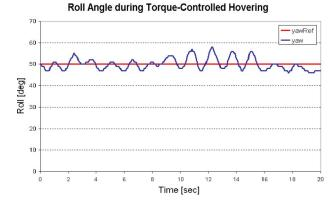
Fig. 13. Roll angle captured during autonomous hovering with torque roll control.
