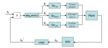
Fig. 3. Block diagram of three compensators for roll, pitch, and yaw.
