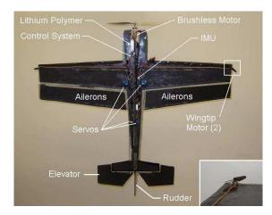
Fig. 12. Two dc motors are added on each wingtip to counter the motor's reactive torque. (Inset) Zoomed-in view of the wingtip motor.
