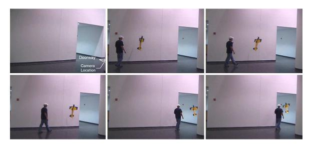
Fig. 18. Hybrid MAV autonomously follows the exterior wall of the building until detecting an open passageway. It then traverses the doorway to gather reconnaissance inside the building.
