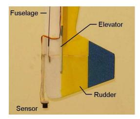
Fig. 14. Mount was created for the sonar sensor so that it would not interfere with the elevator and rudder control surfaces.
