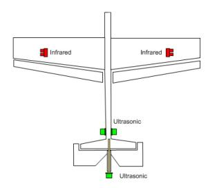
Fig. 17. Infrared sensor is mounted on each wing pointing out from the fuselage. Also, an ultrasonic sensor is mounted at the base of the fuselage pointing outward. This is so the propeller wash does not affect the sensor reading.
