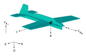
Fig. 4. Vertical vector in the reference frame is shown along with the *x*-axis vector in the body frame.
