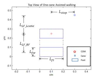
Top view of one-cane assisted walking showing variables Fig. 1
